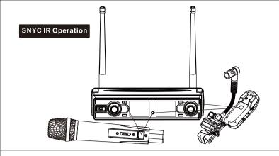
SNYC IR operation shows as above picture. Boot up receiver, and then long press IR button for 3 seconds till the IR indicator flashing and transmit IR signal, meanwhile, boot up microphone and keep ts IR window close to receiver's. Same frequency will show on microphone and receiver at the same time when IR SNYC successfully, and RF signal will show on LDC on receiver.
