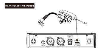
See below RECHARGEABLE picture, use charge cable to connect (17) and saxophone tranmitter's rechargeable port to recharge. When fully charged it will be cut off automatialy
